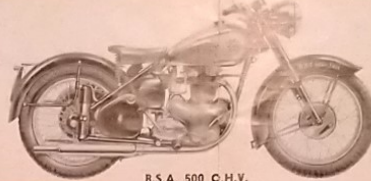
B.S.A. 500 C.H.V. Model A7 Star Twin Now with redesigned engine as Model A7, but with slightly higher compression ratio, the B.S.A. Star Twin offers brilliant performance, whilst the plunger type rear suspension ensures maximum comfort.
