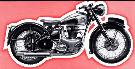
The B.S.A. Star Twin is similar in specification to the Model A7 but incorporates a special camshaft, has a higher compression ratio, a large bore carburetter and an 8 in. front brake—features which combine to give it that brilliant performance which the enthusiast demands.
