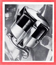
The car-type distributor with automatic advance on the coil-ignition C models is a feature which ensures instant starting and ideal running conditions at all times.
