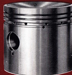
The low-expansion alloy piston with duplex oil control grooves, and slightly concave crown for most efficient combustion.
