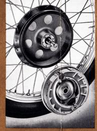
The new 8-inch front breke, with super ribbed shoes for smooth, progressive straight-line stops.
