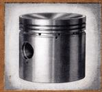
The low expansion aluminium alloy piston, with duplex oil control grooves and slightly concave crown for most efficient combustion.
