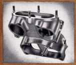
Underside view of the rocker box showing how the airflow channels are designed to follow that of the cylinder head. This also shows the easy access for tappet adjustment.
