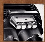
The car-type tappets, with greatly increased bearing areas, giving long life and silent operation, are one of the notable features of the new B.S.A. Golden Flash engine. Note the "siamesed" pairs of tappets providing perfect constant alignment.
