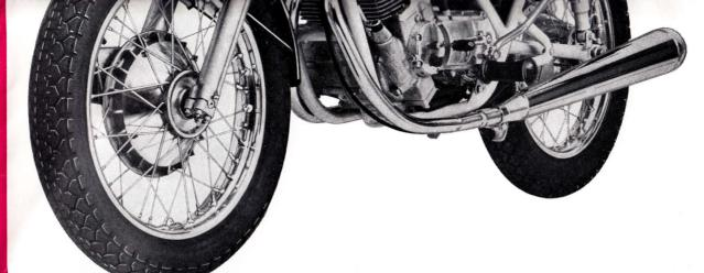
include new slim-line front fork conical hubs, 8" front brakes with 2 leading shoes, 7" rear brake with single leading shoe, front and rear blinkers, new 'megaphone-type' silencers, cushioned instruments and headlamp, dual switch consoles.
